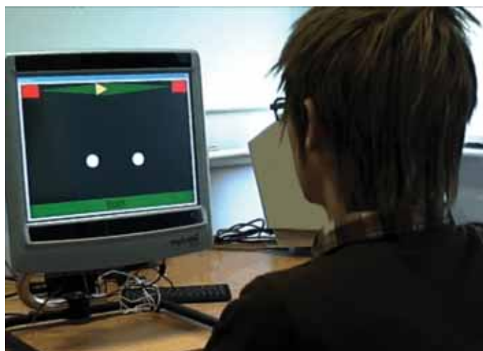
Setting up an eye gaze system – the image on the screen confirms that the camera can see a user’s eyes and that he is the correct distance from the screen
